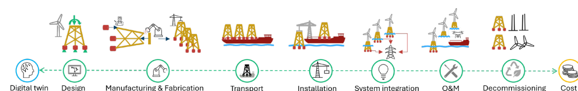
Figure 2: Illustration of the offshore wind value chain – jacket substructure as an example (prepared by Xiaobo Ren, SINTEF)
