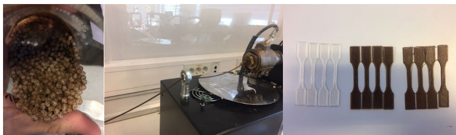
Figure 1: Left) PLA/lignin pellets. Middle) Extrusion of PLA/lignin filament. Right) 3D printed dogbones of PLA and PLA/lignin biocomposites.
