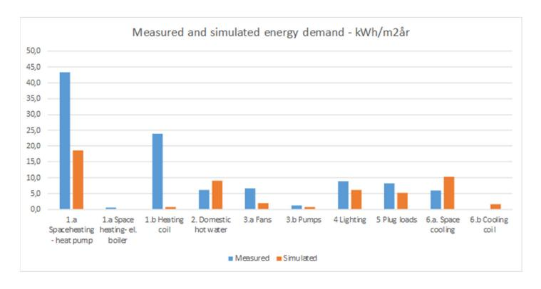
The high net energy use for space heating, ventilation heating and fans is mainly due to a fault after a fire rehearsel, so the ventilation system was running 24/7 a large part of the heating season. Also the integrated heat pump in the AHU is not working according to the intention.
