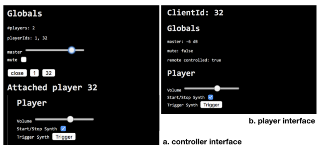
Figure 9: Interface of the (a.) controller and (b.) player clients of the Todo(Noise) application. Here, the controller duplicates the interface of the player with id 32, allowing for remote monitoring and control of this particular client.
