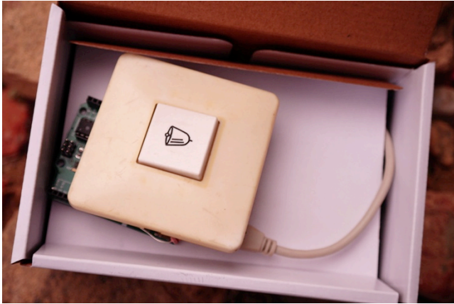
Figure 10. The bell of the Ring the Web! project, using an RPi Zero.
