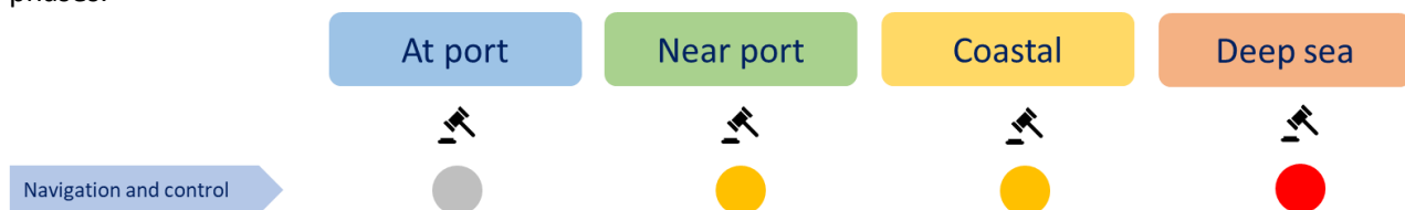
Figure 17: Regulatory feasibility for navigation and control for an unmanned cargo ship. All phases except deep sea are regarded as domestic/national.
