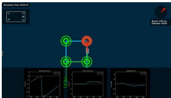
Snapshot of RL-NMPC controlling the milliAmpere 1 on the 8-corner test in a simulation environment, under the presence of wind.
