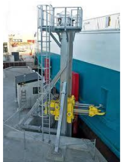
Figure 3: Mooring solution that does not require ropes. Courtesy: MacGregor.
