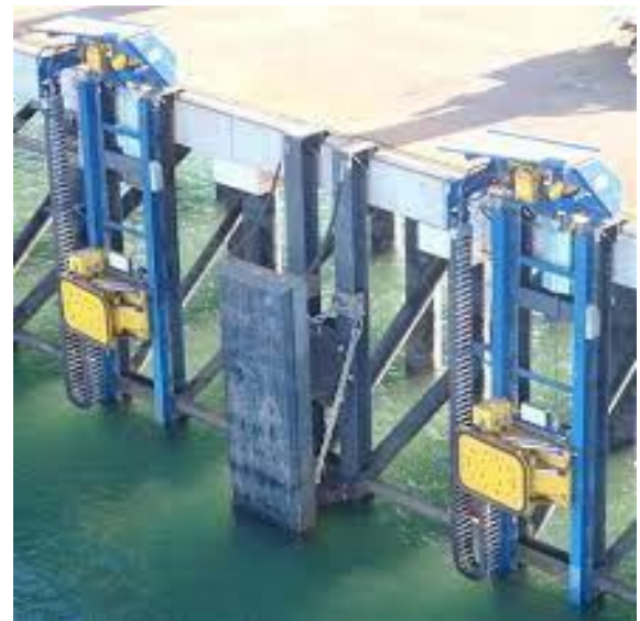
Figure 8: MoorMaster in front of quay. Courtesy: Cavotec.
