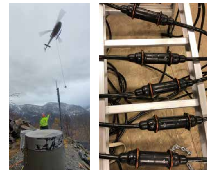
Figure 18 (R). 3-component borehole geophones re-equipped with centralizers to stabilise them within the borehole to improve signal to noise levels.
