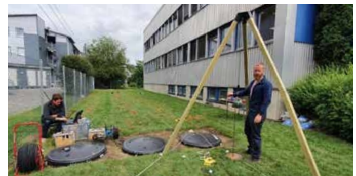
Figure 12. Acquisition of DAS and geophone data at the NOR-FROST test site behind the NORSAR office building in Kjeller.
