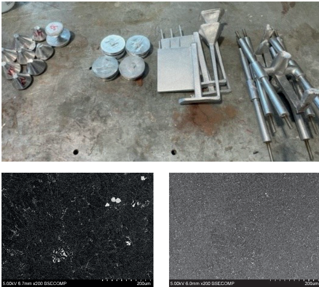
Figure 1 AlSi10MnMg with incinerator bottom ash (IBA) aluminium. Top: cast samples, Left: Microstructure with 30% added IBA, Right: Microstructure of reference sample.
