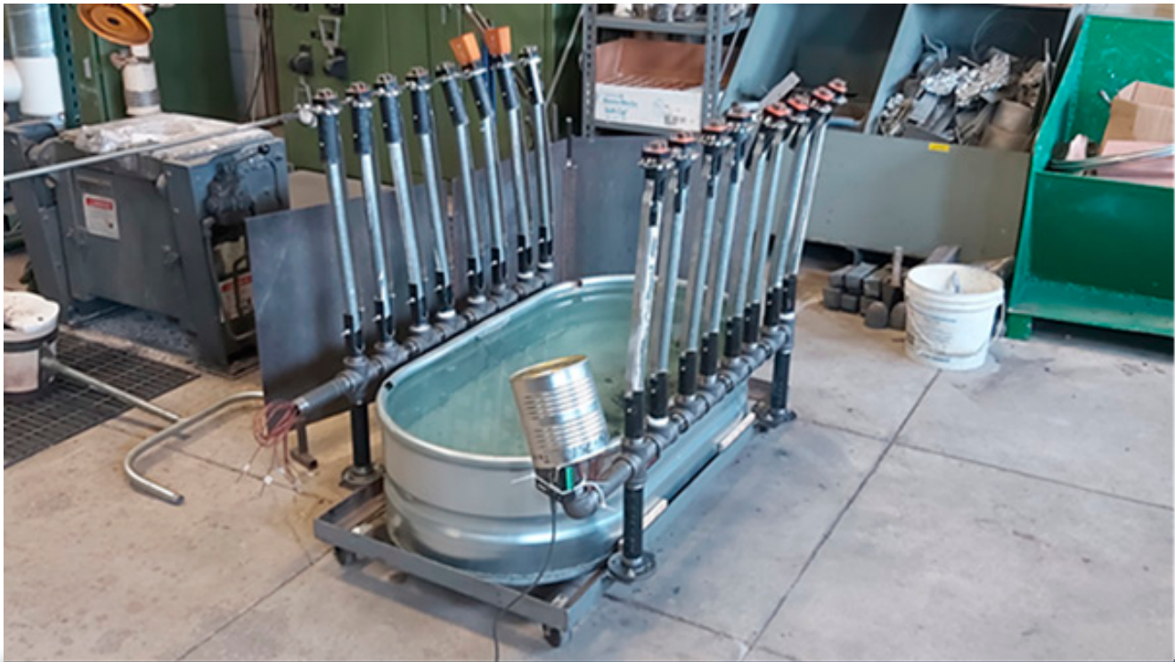
The image shows the setup of the quenching experiments carried out by A. Bugten at MTU. Cooling cups with integrated thermocouples are filled with cast iron. The cups are then released into the water-filled container at appropriate temperatures.
