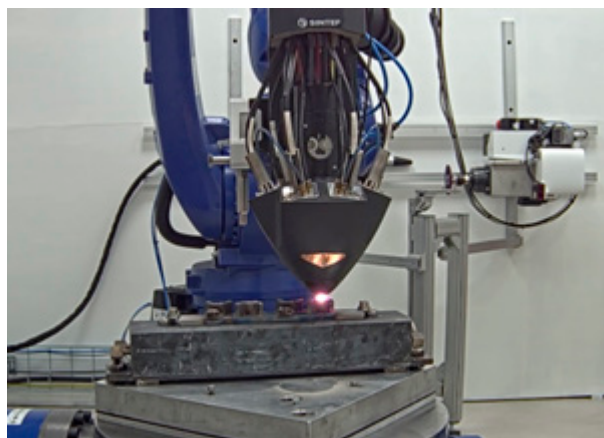
Figure 6. Experiment setup for Dr. Hassel's PhD work, i.e., laser DED of duplex steel.)
