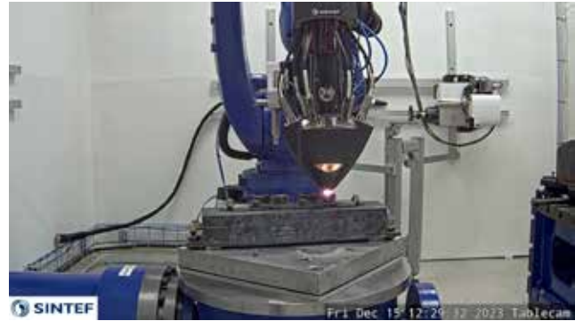
Example of laser DED of Duplex specimens.
