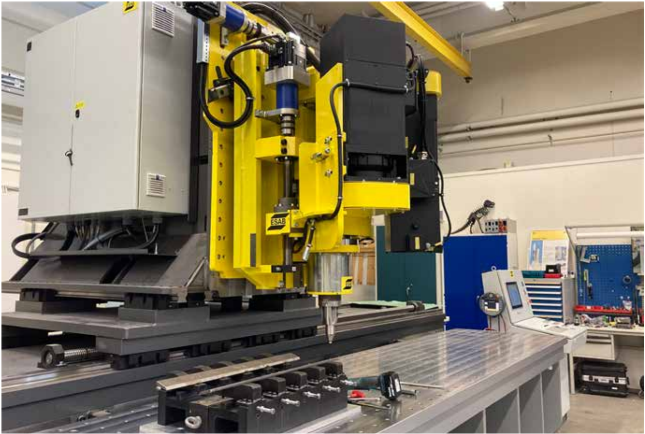
Friction Stir Welding equipment installed at Raufoss, SINTEF Manufacturing.
