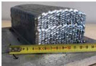
Figure 2a) WAAM material (added TiC particles, screw extruded, and wire arc welded).
