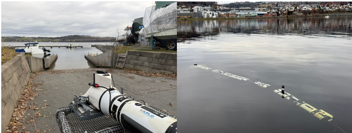
Figure 13: UHI sensor on the snake robot Eely.
