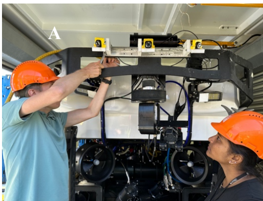
Figure 16: A) Preparation of ROV Minerva with a stereo camera setup. B) Vehicle tuning and control in the lab of RV Gunnerus.
