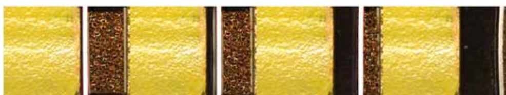
Fig.2 Pictures of a 20 mm thick galvanized (Cu) foam during the crushing process, taken every 0.33 ms
