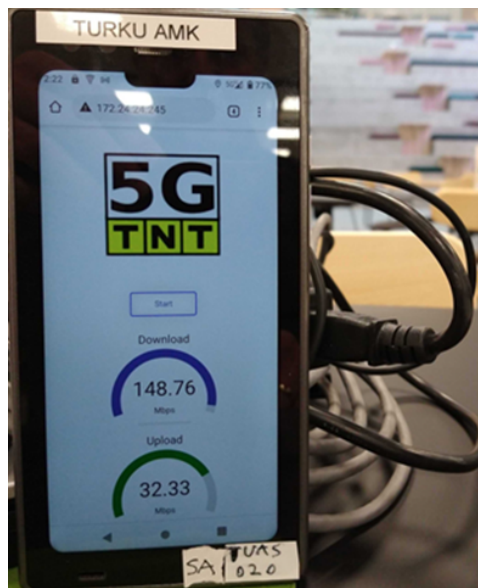
Figure 2. Measurement device for the 5G measurements.
