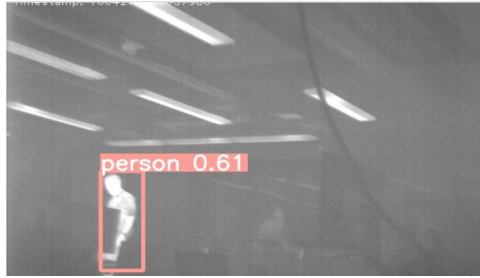
Figure 4. An example of a person detected from the thermal camera image. The confidence level of the detection is 61%. This rather low confidence level occurs due to the partial occlusion of the person.
