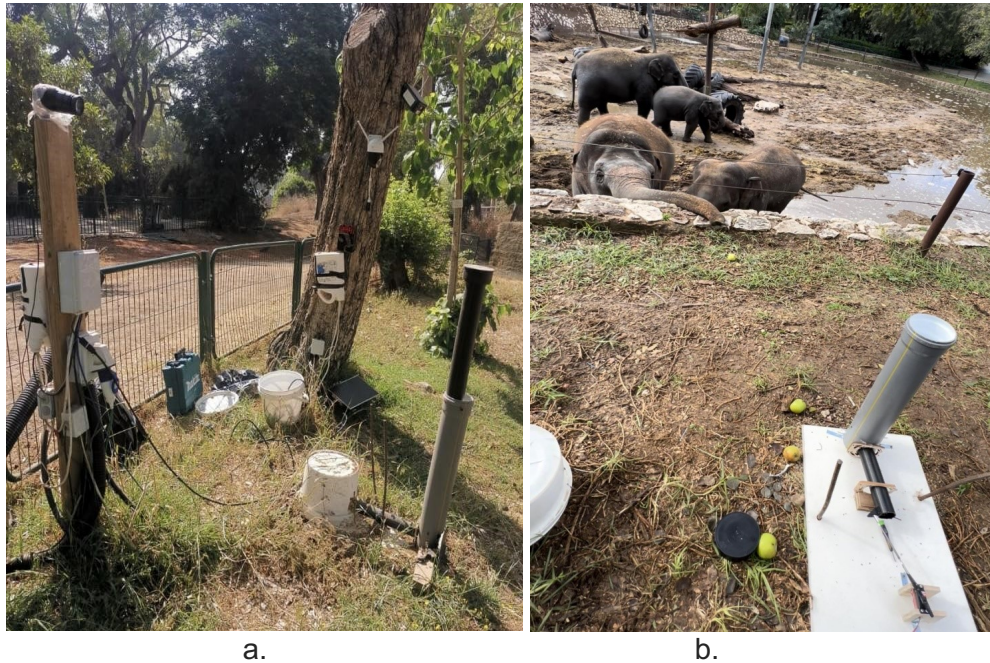
Figure 2. EleProje – Elephant monitoring system. Figure 2a. System components deployment. Figure 2b. Mechanical fruit reward sub-system.
