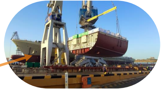
Pre-outfitted blocks shipped for assembly
