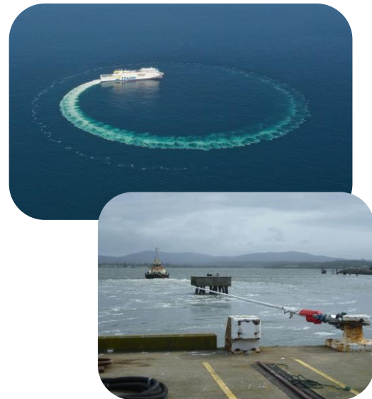
Turning Tests and Bollard Pull Testing
