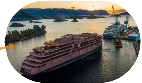
Ship already launched, towed for outfitting and painting
