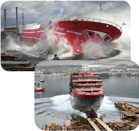
Side and Slipway Launching
