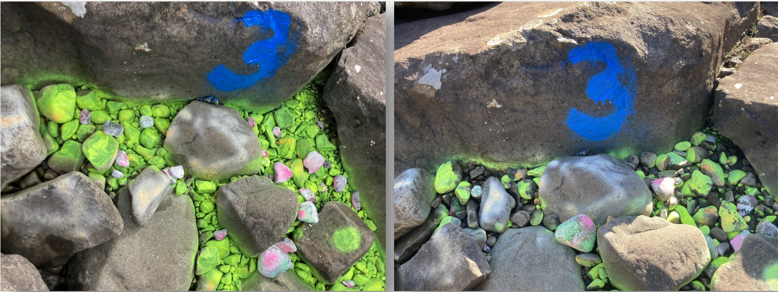
Pebble and cobble patch pre (left) and post (right) a 98 cumec spill - Derwent River downstream of Wayatinah Lagoon
