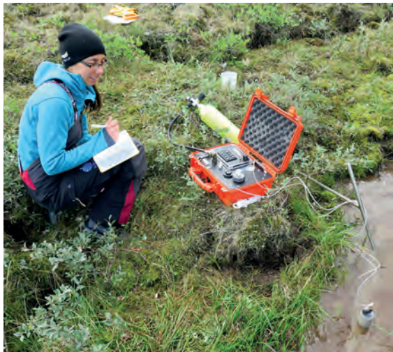
Measurements of the critical shear stress in a small gully at the Inuit village of Salluit located north of the province of Quebec in Canada
