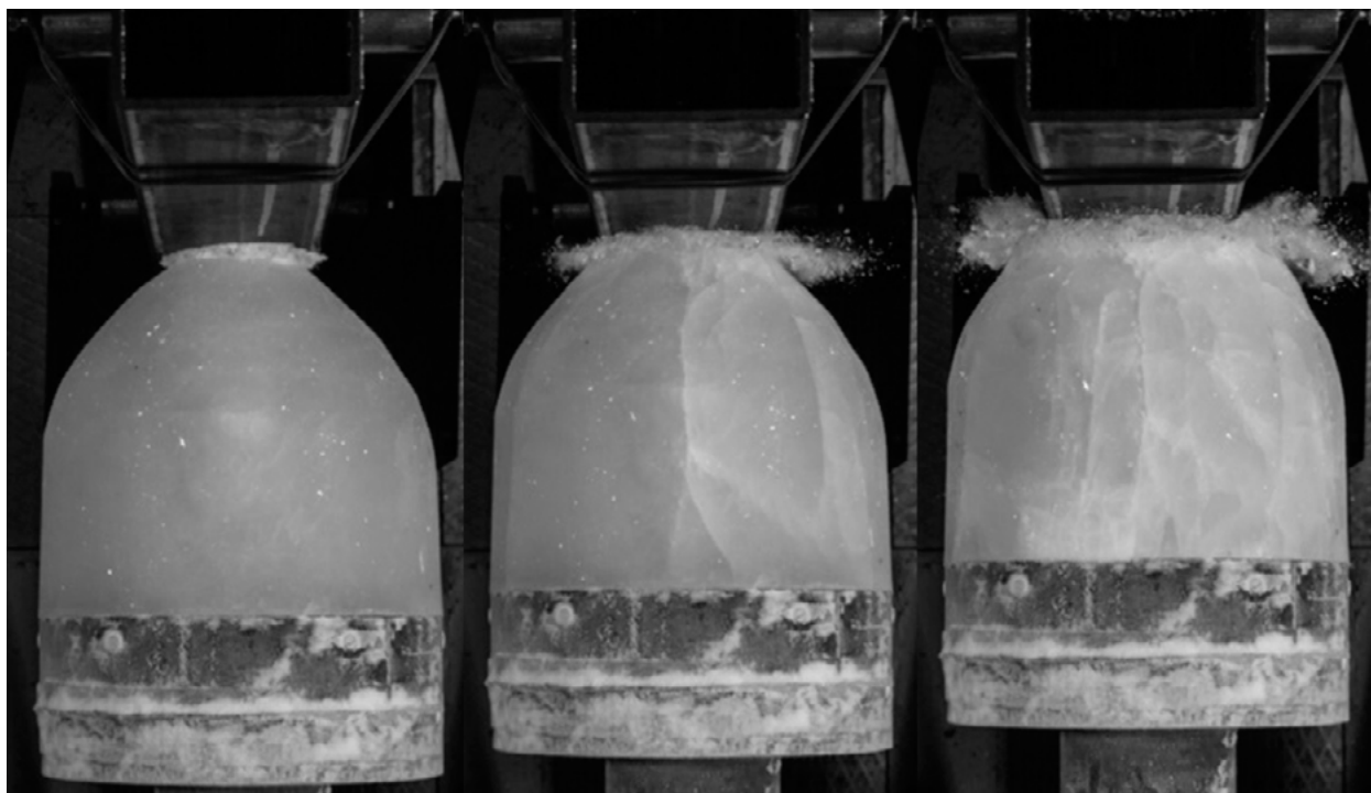
Figure 29. High-speed video of the ice impact experiments.
