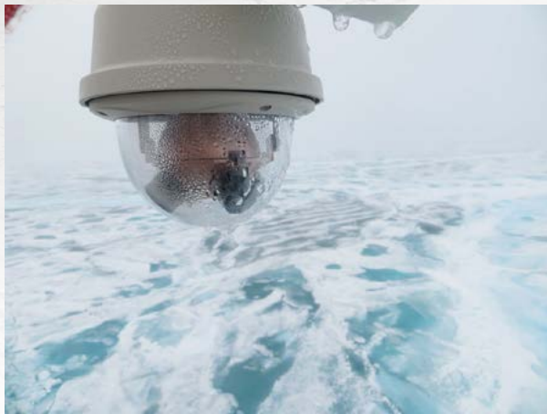
Figure 31: One of the 360CamSys camera domes, showing some unfortunate fogging. Courtesy: Bjørklund et al. (2013).
