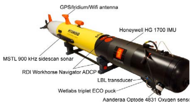
Figure 35: The NTNU REMUS 100 AUV used in SAMCoT research (Norgren and Skjetne, 2014).
