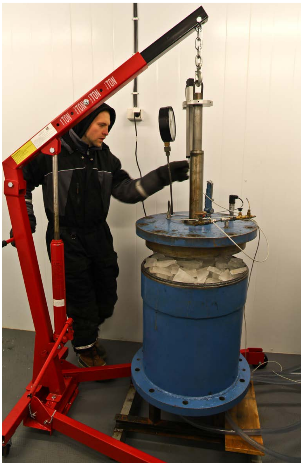
Figure 17. PhD candidate Sergej Kulyakhtin preparing oedometer experiment in the NTNU cold lab.
