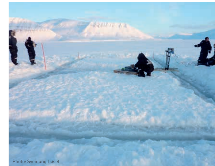
Figure WP4_4. A trial campaign in the field to acquire the fracture properties of sea ice.
