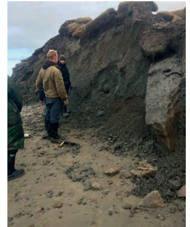
Figure WP6_4 Sampling from different parts of the coastal sediments at Baydaratskaya Bay for later laboratory work.
