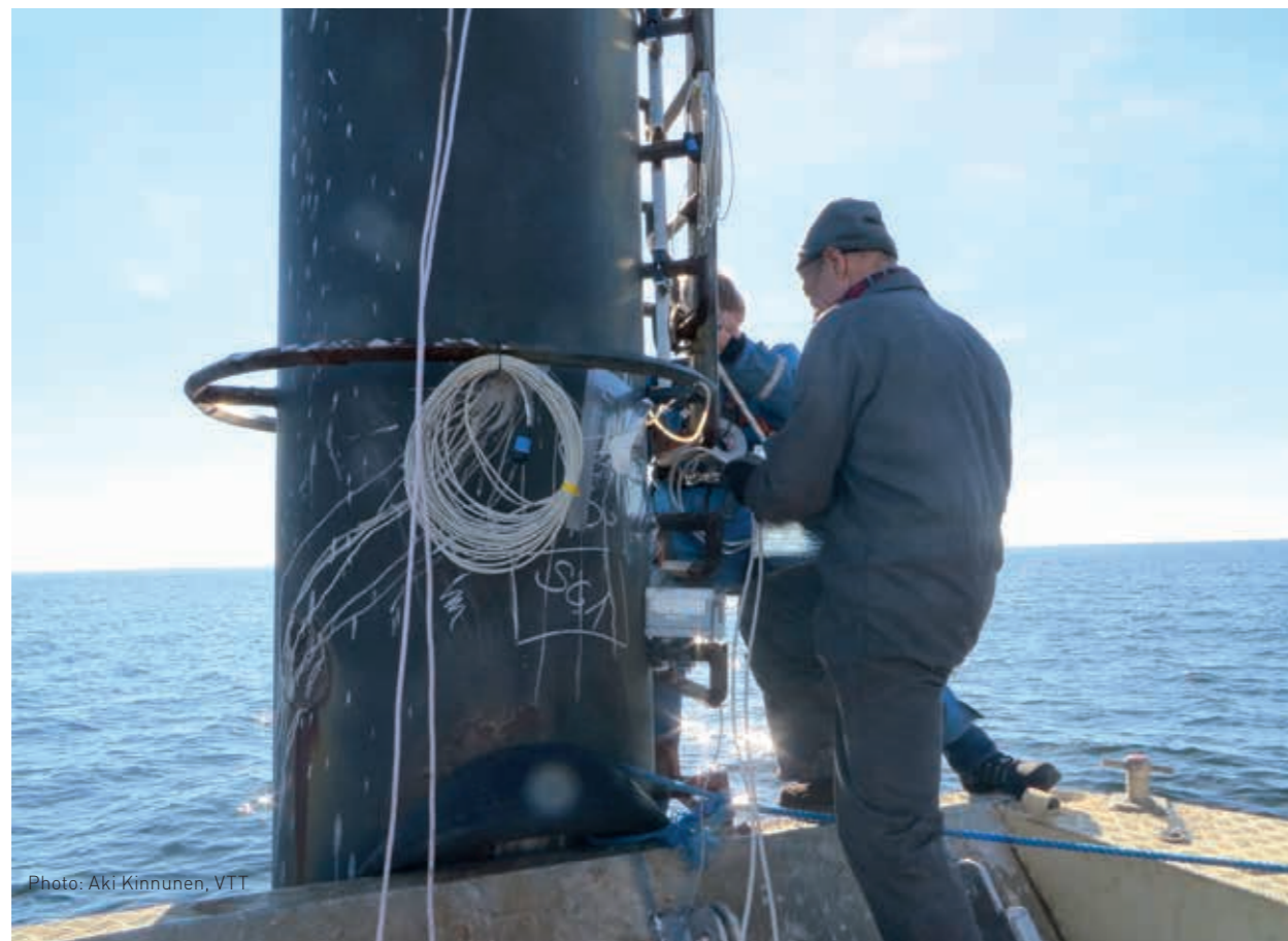
Figure WP3_1 Mauri Määttänen and an VTT Engineer installing strain gauges to the Hanko-1 channel marker in the Gulf of Finland.
