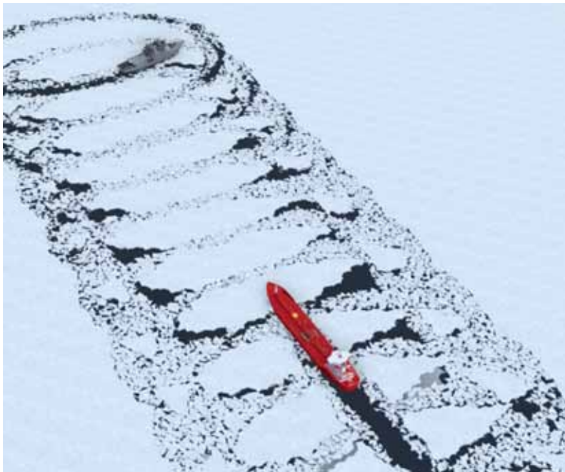
Fig. 12: Real-time simulation of Ice Management (NTNU/SMSC).
