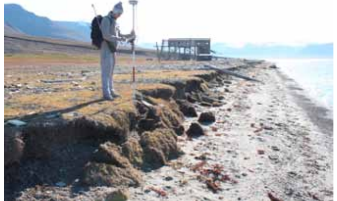
Fig. 13: Survey on a beach bluff edge in central Spitsbergen. It displays the uneven edge and a small detachment of vegetated soil. An old coal depot can be seen in the background.
