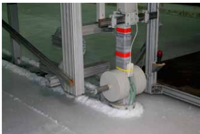
Fig. 7: The model structure: a) Forced movement technical drawing and b) the structure harmonic motion through level ice.
