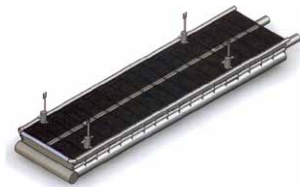
Fig. 21. One section of the floating jetty.
