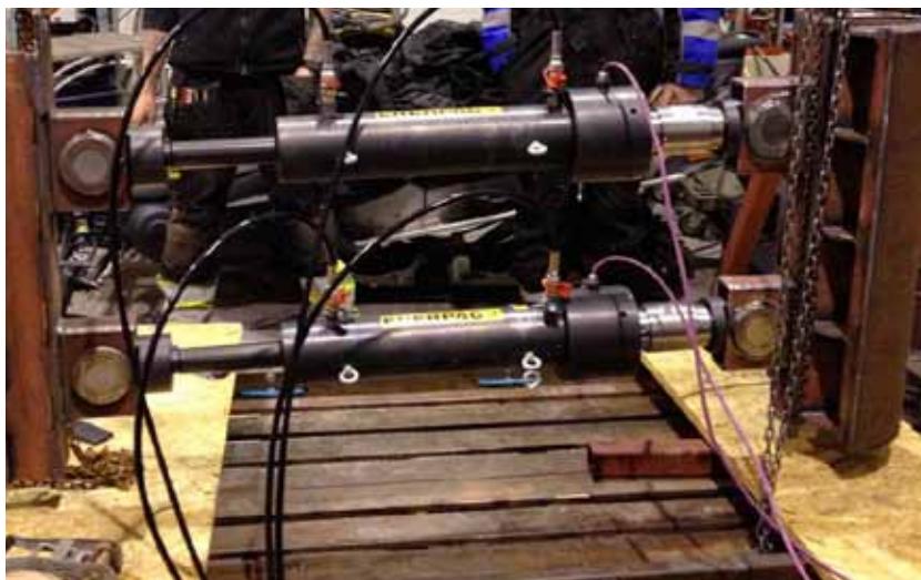
Fig. 2: The new indentation rig for in-situ ice testing.
