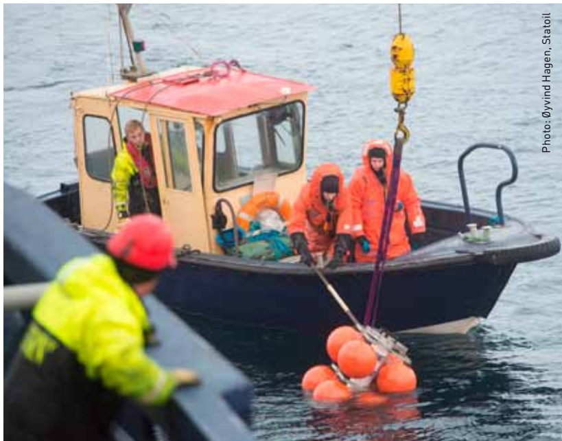
OATRC2012 cruise members deploying Ice Profiling Sonar (IPS) and Acoustic Doppler Current Profiler (ADCP) mooring.
