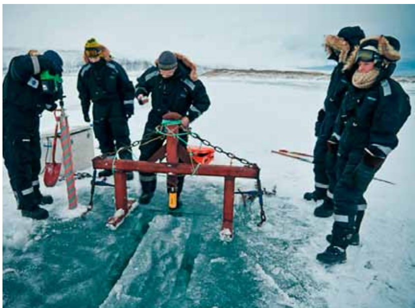
Fig. 3: Students in AT-332 perform an in-situ beam test in Svalbard.
