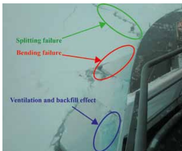
Fig. 9. Waterline processes (splitting, bending and ventilation effects).
