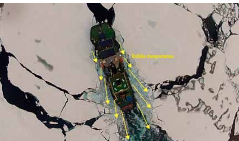
Fig. 13. Bird's-eye view of the icebreaker Oden and the transport of broken ice, indicated by yellow arrows.
