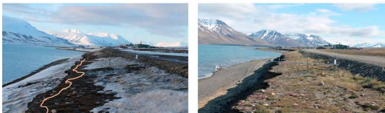
Fig. 35. Photos shot with a time lapse digital camera at Vestpynten. The photo to the left was taken on 23 May 2012, while the photo to the right was taken 12 July 2012. The orange line represents the edge line position in July (from the work of PhD candidate Emilie Guegan).
