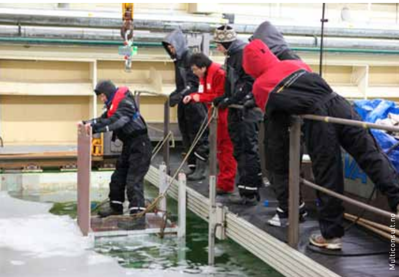
Buoyancy box used to measure ice parameters and video capture ice behaviour characteristics.
