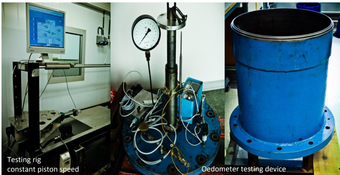
Photos taken by A. Pustogvar during the shear box and oedometer tests.
