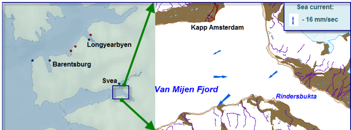
Example of sea currents speeds measured in Van Mijen Fjord on the phase of maximal tide
