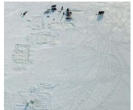
Fracture tests of ice floes with different orientations.
