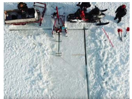
Kink tests (a drone view from above showing the crack path highlighted with red markers)
