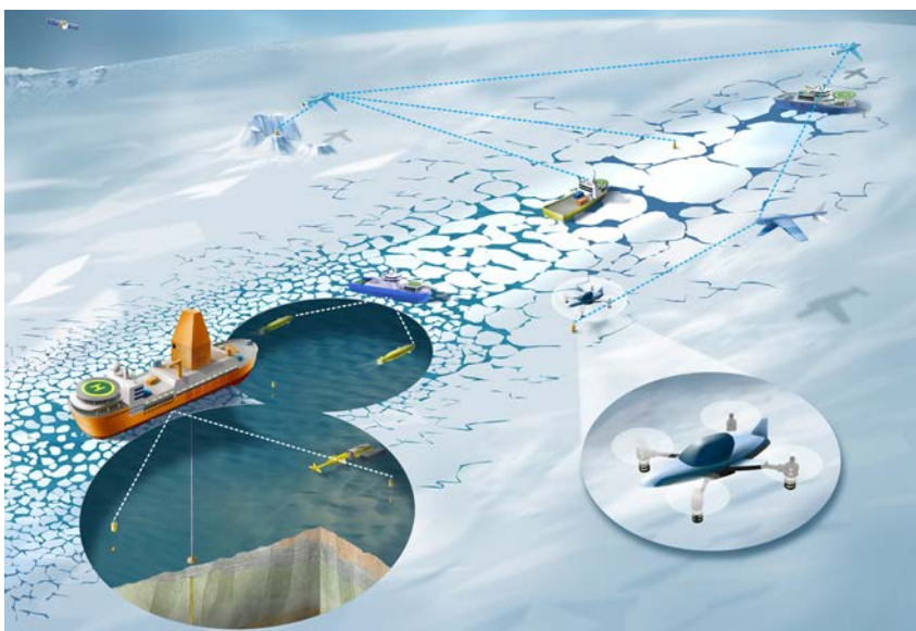
Example Ice Management operation with a protected vessel, 3 icebreakers working upstream the ice drift, and several ice surveillance platforms.
