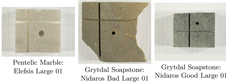
Fig. 4. Photos of some stone slabs used in the accelerated erosion experiments.
