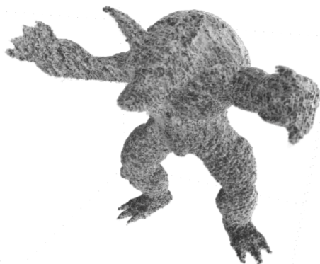
Figure 5: A 3D volume obtained by the voxelization of the "Armadillo" mesh, which is subsequently flood-filled starting from several seed points. Three cross-sections of this volume are depicted in figure 6 and reveal that the considered 5 \times 5 neighborhood in the sampling is large enough to make the Voronoi cell transitions less apparent.
