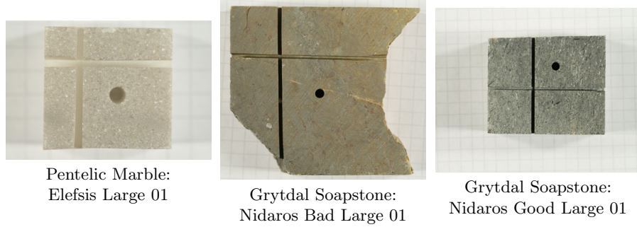
Fig. 6. Photos of some stone slabs used in the accelerated erosion experiments.
