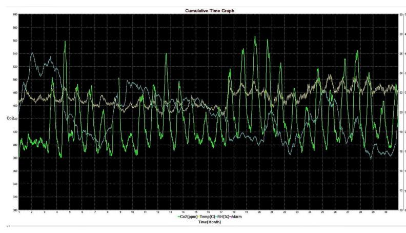
The variation in Temperature, RH and CO<sub>2</sub> level in November 2014 in the lab where the acid weathering was carried out.
