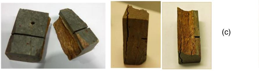
(a) Close up images of NB stones in acid mixtures in the first round with increasing cracking and enhanced eroding of iron sulfide, dolomite and iron oxide rich site (b) Iron oxide rich localities emerging and eroding faster than other parts in NB stone in sulphuric acid solution. They got yellowish\orangish in colour. The cracking gets enhanced leading to volume expansion and eventually detachment. The white precipitations are gypsum confined to selected localities.
