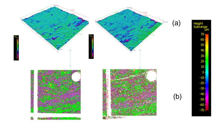
3D laser microscope images of the surfaces of NB stone in nitric and sulphuric acid solution before weathering and after second round (from left to right) (a). The greater loss at the edges compared to the inner parts is observed. The mineral map of the same stone above from QEMSCAN at low magnification (100x100 micron resolution).
