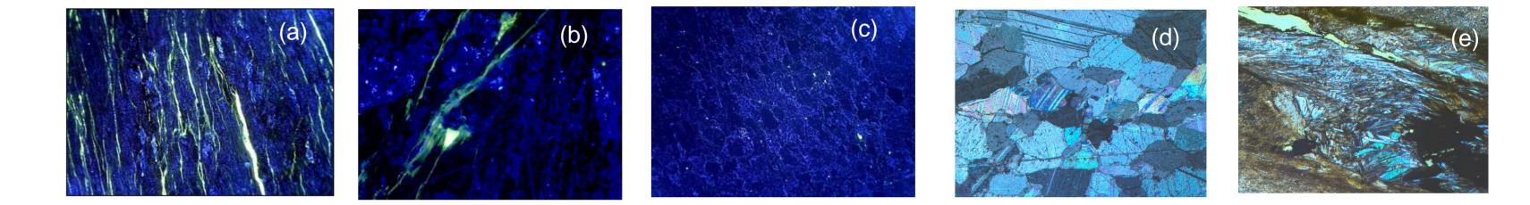
Fluorescence imaging of thin-section samples prepared by embedding in a resin containing fluorescent compound. The cracks and fissures are
