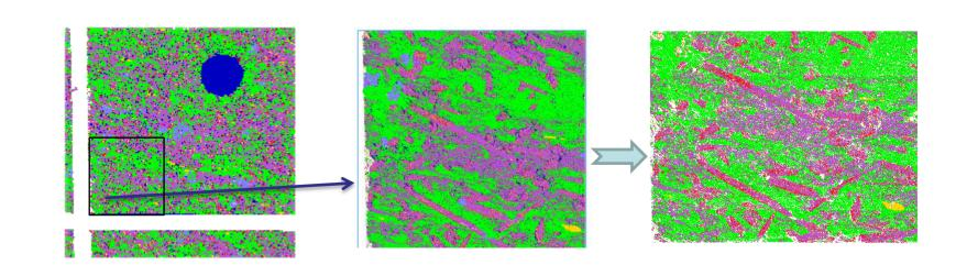
The mineral map of NG stone in a mixture of nitric and sulphuric acid solutions at low magnification (100x100 micron resolution) left and high magnification (10x10 micron resolution) the middle and the right. The comparison is between the stone composition before the accelerated and after the second round. Loss of dolomite and conversion of actinolite – tremolite elongated grains due to gypsum formation are indicated. The chlorite appears less affected by the acid action.
