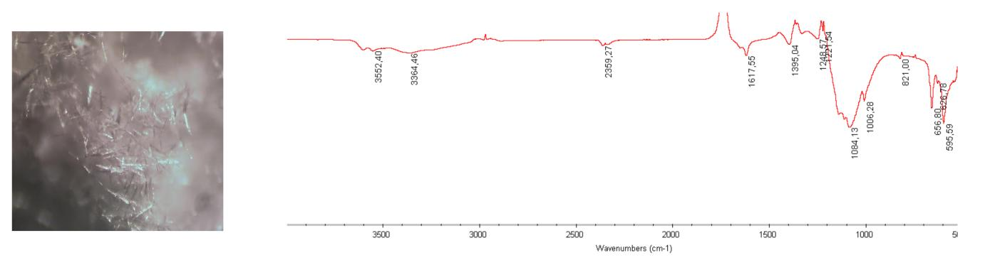
Microscopic image of the crystals formed up on drying of the leachate from sulphric solution in which Elefsis marble stones were immersed. The cyrstals are identified as gypsum from their IR spectra (a). The spectrum of gypsum from the acid mixture chamber containing NB stones (b).
