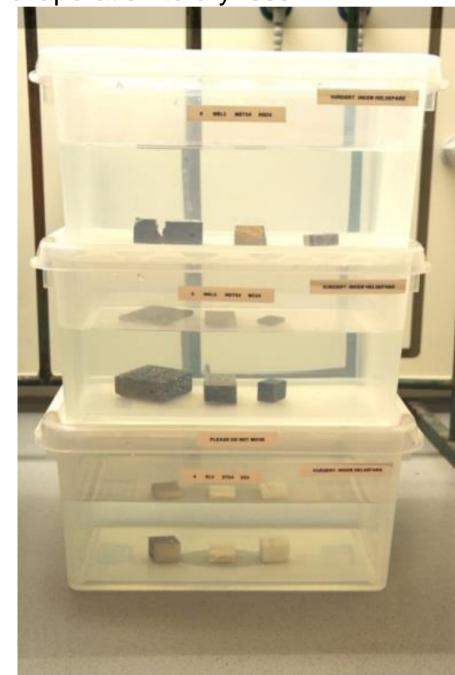
During immersion of the three sets of samples stones in separate acidic solutions
