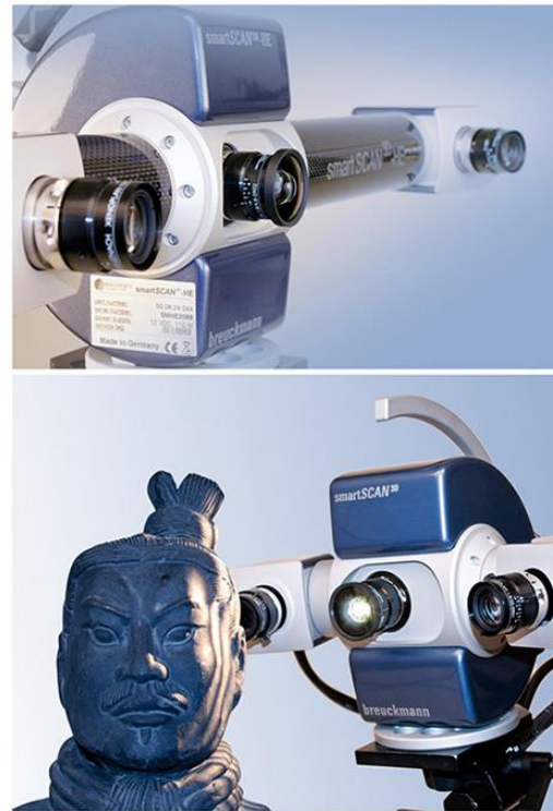
Fig. 7 - A smartSCAN 3D white light scanner with three triangulation angles. Left: the asymmetric placement of the cameras relative to the projector allows for triangulation angles of 10° and 20° for 3D data acquisition using white light scanning as well as 30° triangulation angle for stereo-metric measurements. The triangulation base length ranges between 240 and 470 mm depending on the field of view chosen for a scanning project (right).
