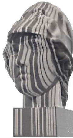
Figure 3. Shape from structured light 2
