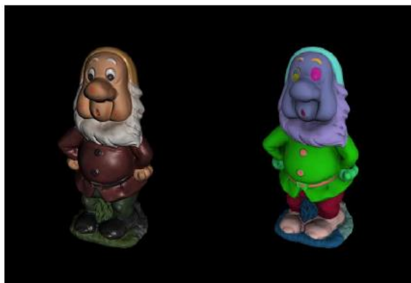
Figure 21. 3D COFORM: first result of reflectance estimation from video flows, a rendering of the object with estimated reflectance (left), the clustering of the object, showing all the surface portions with different material behavior (right) 36 .
