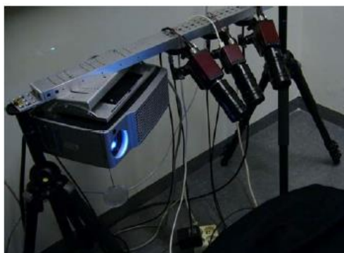
Figure 5. 3D COFORM: the original “in-hand” scanner setup 36 .
