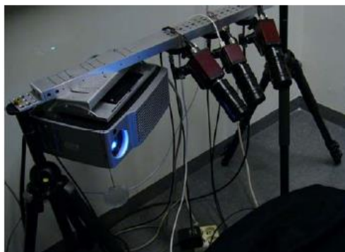
Figure 12. 3D COFORM: The original “in-hand” scanner setup 36 .
