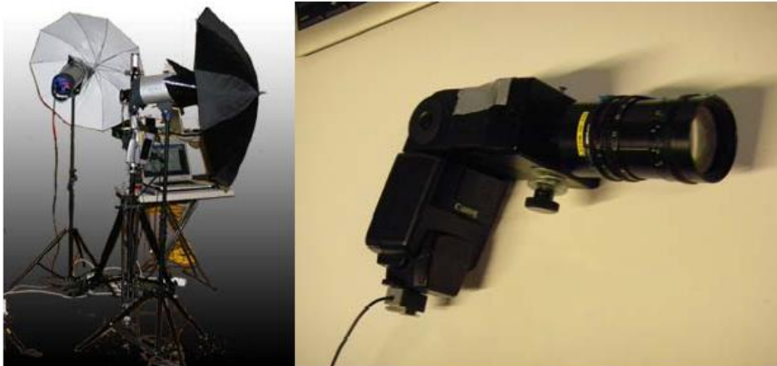
Figure 13. 3D COFORM: The new “hybrid” system. The umbrellas can be attached to the SLR to guarantee diffuse lighting. Right: Flash unit with built-in patterns and lens. When the SLR takes an image the flash fires a pattern on the object 36 .
