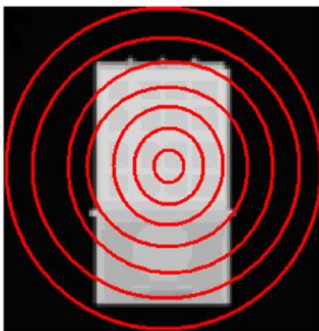
Figure 27. Top elevation of the 3D jeep model shown in Figure 26 partitioned by several concentric circles 51 .
