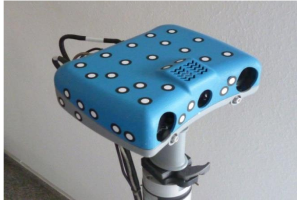
Figure 10. 3D COFORM: Breuckmann hand held 3D scanner.
