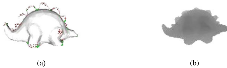
Figure 47. (a) Salient points must appear on the contour of the 3D objects for a 2D view to be considered as a ‘salient’ view. The contour salient points are colored in green, whereas non-contour salient points are in red, (b) silhouette image 128 .
