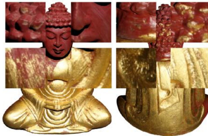
Figure 20. 3D COFORM: achieved quality of an object acquired with the new multi-view dome object acquisition pipeline, employing a 3D reconstruction obtained with the novel structured light method 37 together with BTF reflectance data 36 .
