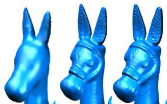
Figure 19. 3D COFORM: quality comparison of reconstruction methods, demonstrated on a metal donkey figurine: visual hull, previously used in multi-view dome (left), NextEngine laser scan (center), novel multi-view dome 3D reconstruction (center) 36 .
