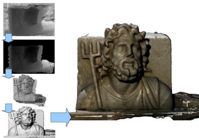
Figure 6. 3D COFORM: automatic mesh generation from ARC 3D depth maps 36
