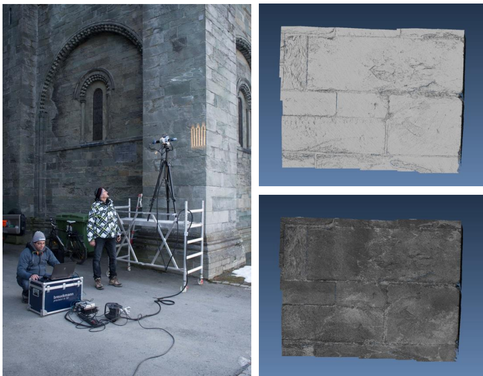
Figure 2. Scanning outside of the north entrance of Nidaros cathedral (left). The result from monochrome texture mapping (lower right image) using sensor imagery provides an added value for documentation and visualisation.
