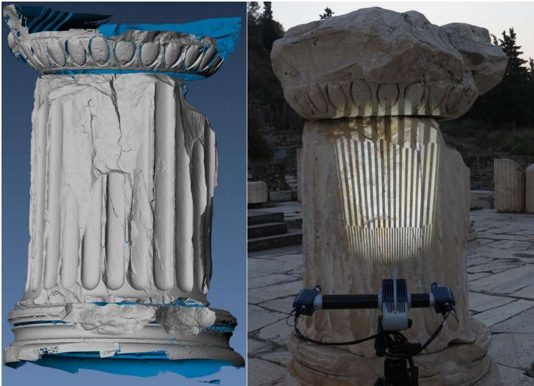
Figure 1. Visualisation of the 3D scanning results from Elefsis in OPTOCAT software (left). Data acquisition with a Breuckmann white light scanning system (right).
