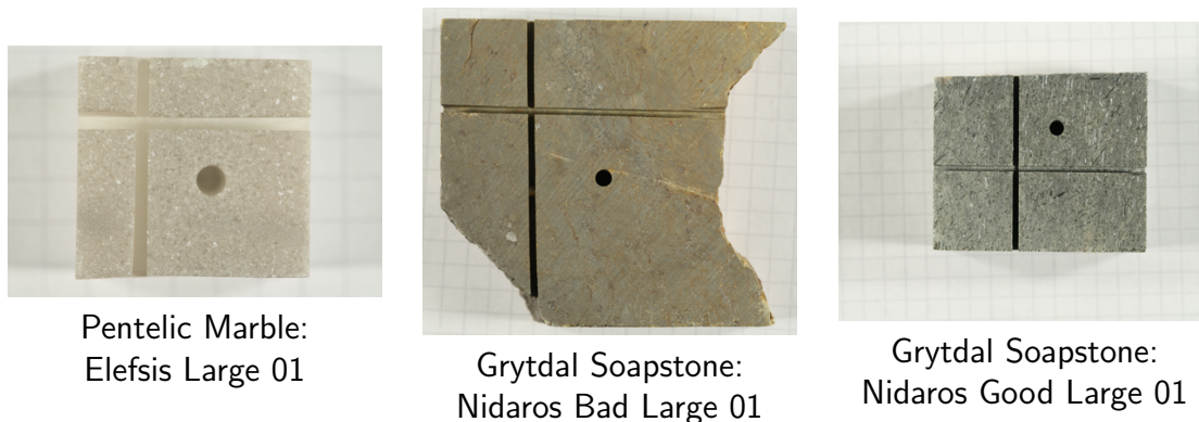
Figure 9: Photos of some stone slabs used in the accelerated erosion experiments.
