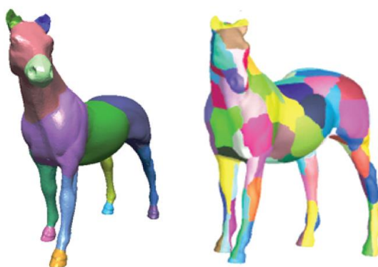
Figure 27: Two different types of mesh segmentation. Left: Part-based segmentation. Right: Surface-based segmentation of the same mesh. Image taken from [112].
