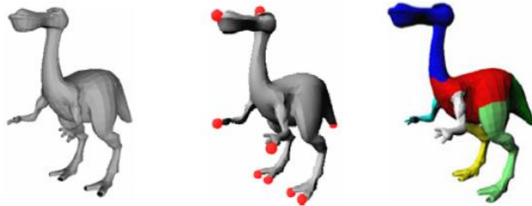
Figure 37: Mesh segmentation guided by critical points. Left: The input mesh. Middle: Critical point selection. Right: The final segments. Image taken from [145].
