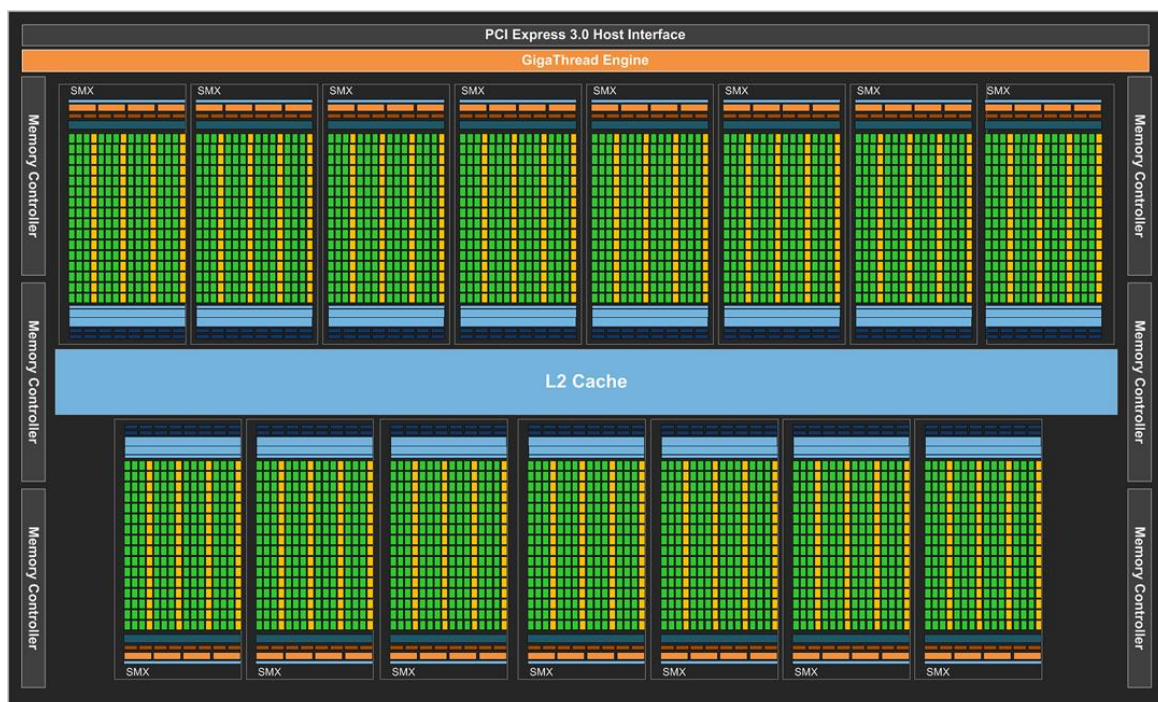
Figure 64: Block Diagram of a modern GPU (Nvidia Kepler Architecture). The chip consists of a large pool of computation cores, shown as green. Memory buffers and cache memory are shown in blue. (Source: NVIDIA Corporation).
