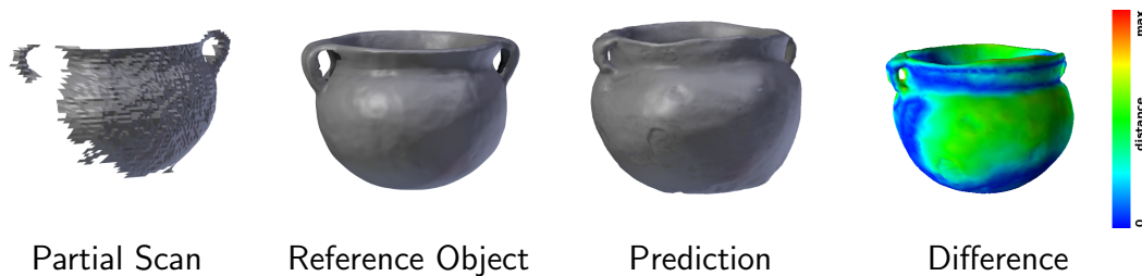
Figure 90: Predictive scanning results on the HM438 object, obtained with Microsoft Kinect V2 for Windows sensor. RMSE = 6.95mm.
