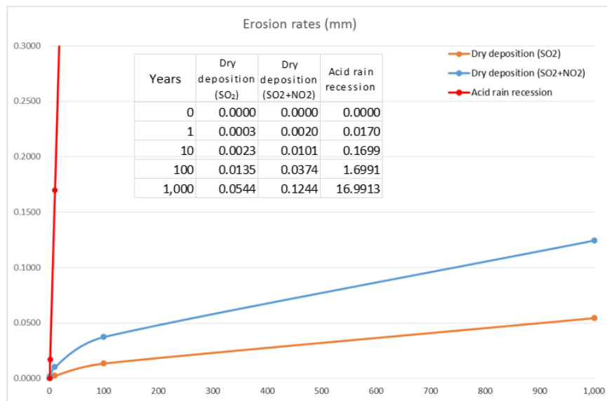
Figure 42: Erosion rates computed on marble under certain environmental conditions for the comparison of the different weathering cases.
