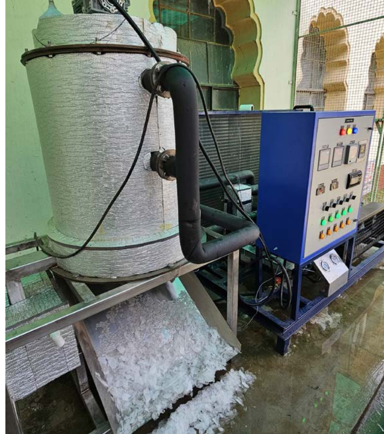
INDEE3 Flake Ice unit (R290) at BITS Pilani India.
