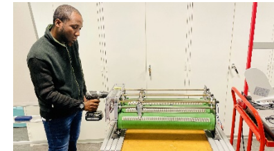
Varying load on the generator
