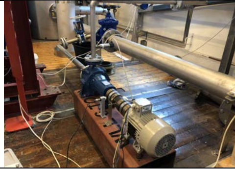
Picture: Small scale pump as turbine experimental setup at NNTU, which has been shipped to UDSM
