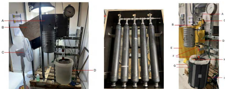
Laboratory setup for testing of adsorption refrigeration cycle with carbon/ ammonia
