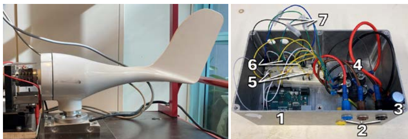
Laboratory setup with wind generator and Arduino based load switching
