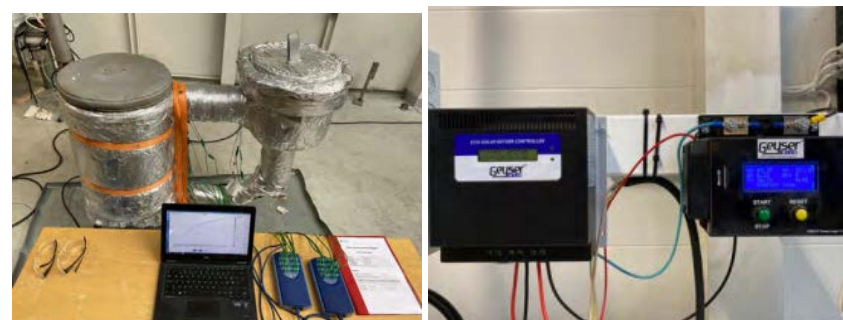
Laboratory setup for testing of PTC heating element in dual tank solar cooker
