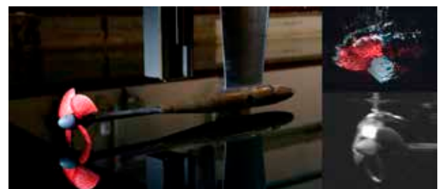
Figure 15: Test set-up and snapshots from propeller ventilation model tests by Anna Kozłowska.
