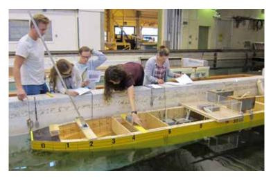
Figure 1: (Kristin Lauritzsen, NTNU): Master students conducting experiments in the towing tank.
