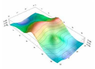
Figure 7: Free surface elevation resulting from a turbulent wave-current interaction. These waves were initially long-crested, but after 5 wave periods, they have become short-crested as a result of the turbulent wave-current interaction.
