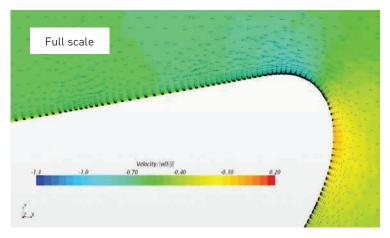
Figure 15: CFD simulation result of the flow around Duct 19A at both model and full scale. The separation zone on the outside is clearly shown at model scale; however, there is no flow separation at full scale.
