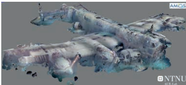
Figure 21 (Stein M. Nornes, NTNU): Photogrammetry model of the wreck of the Halifax bomber aircraft.
