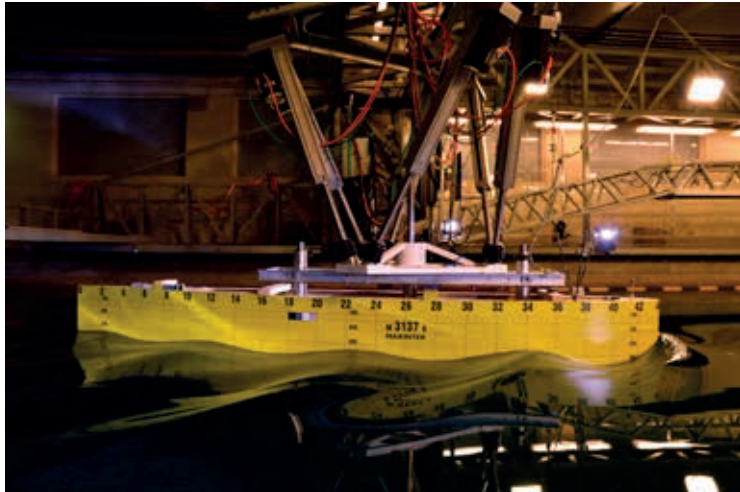
Figure 12a (Jarle Andre Kramer, NTNU): Validation experiment for drift-induced forces.
