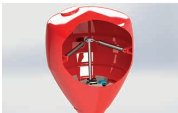
Figure 17: CorPower Ocean's wave energy buoy, with three WaveSpring cylinders connected between the buoy hull and the centre rod.
