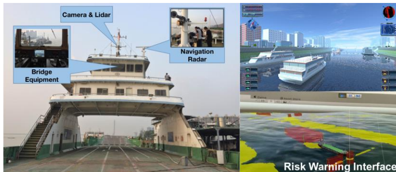
A parallel 3D simulation system has been developed on a ferry ship in the Yangtze River, China.
