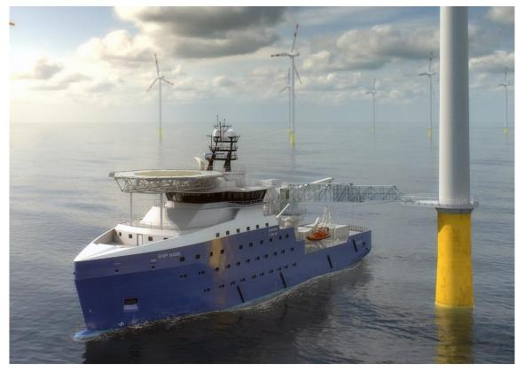
Automated operation between wind turbine landing points, integration with gangways
