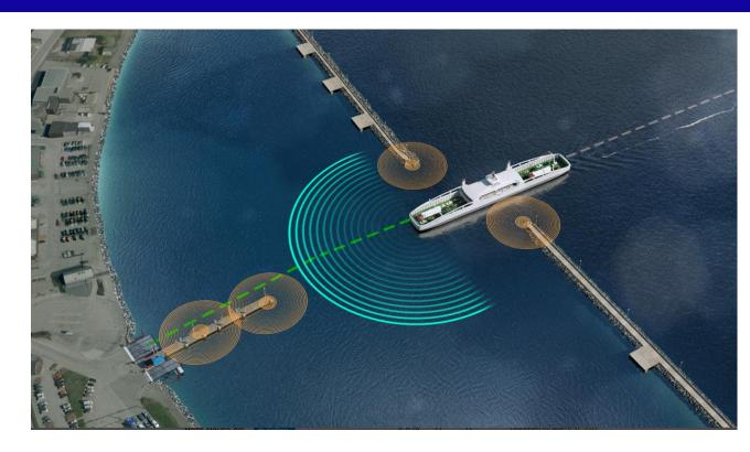
Automatic crossing and docking of ferries, by combining propulsion & DP controls
