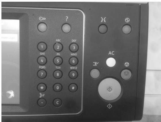
Figure 7: Physical control interface
