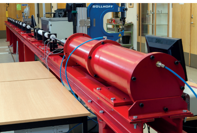
Figure 13 – Split-Hopkinson pressure bar. Photo: Ole Morten Melgård
