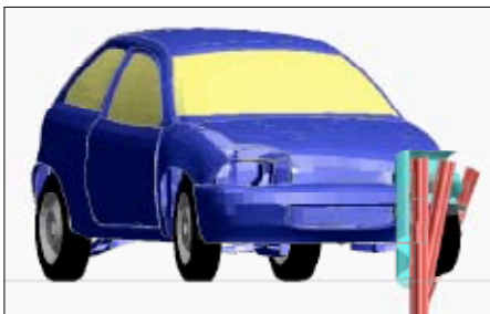
Figure 16 - Impact between guardrail and a vehicle.
