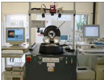
BUP-machine with a camera system for field measurements
