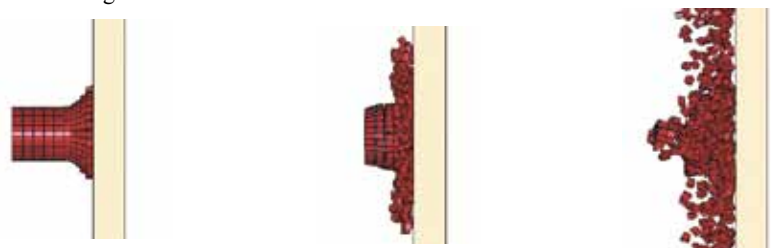
Figure 8 - Comparison between an experimental test and a numerical simulation of a Taylor tests using a steel projectile hardened to HRC 53.
