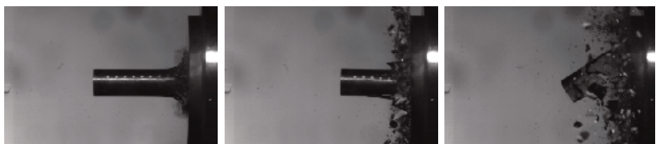
Figure 7 - Sequence of plots showing the deformation of the AL-6XN plate after impact of C-4 and saturated wet sand at stand-off distance of 150 mm.
