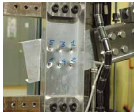
Figure 21 – Behaviour of assemblies using aluminium rivets.
