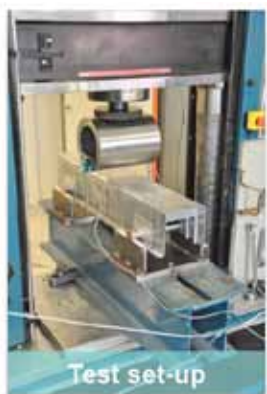
Figure 3 – Bending tests of HPDC component. The test set-up is shown to the left, whereas the right diagram shows the scatter of the force-displacement curves between parallel tests.
