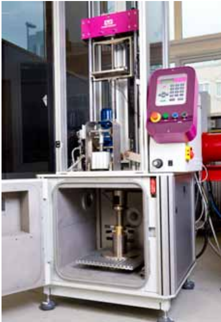
Figure 34 – Droptower impact system. Photo: Ole Morten Melgård
